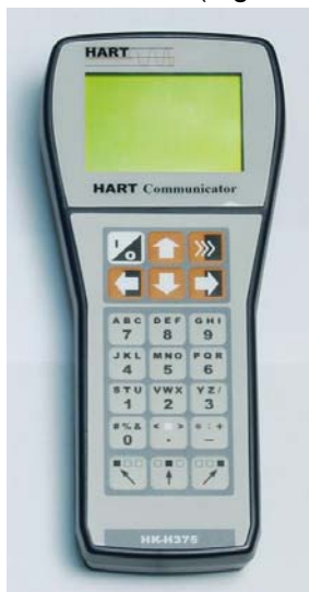
Figure 1 HK-H375A HART Hand Held Communicator
