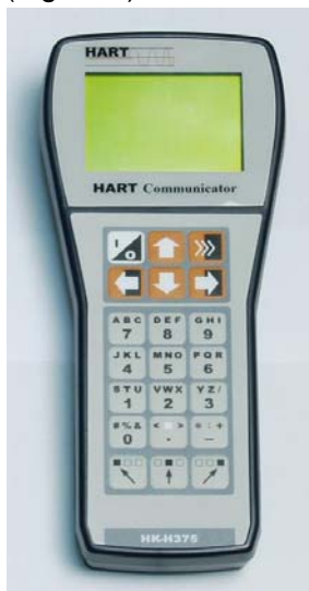
Figure 1 HK-H375A HART Hand Held Communicator
