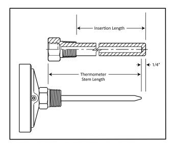
For more detail on thermowell selection see the Tel-Tru Thermowell Selection Guide. https://www. teltru.com/images/catalogs/TW1000/TW1000.pdf
