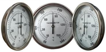
To reduce parallax-error, it's always best to read an instrument from directly in front if possible.
