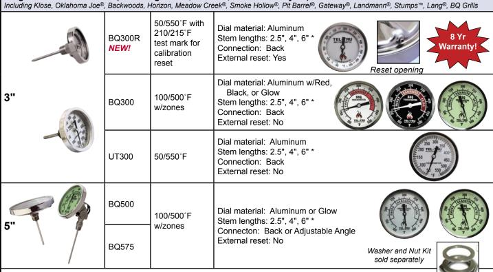
Installation: The above models have a 1/2" NPT connection which threads into a welded coupling or installs into a 7/8" diameter hole with washer and nut (sold separately p/n 4903101). A minimum of a 4" stem is recommended to ensure that the bimetal sensor is a fully immersed into the cooking chamber. \* Select a 6" stem for an insulated cooker.
