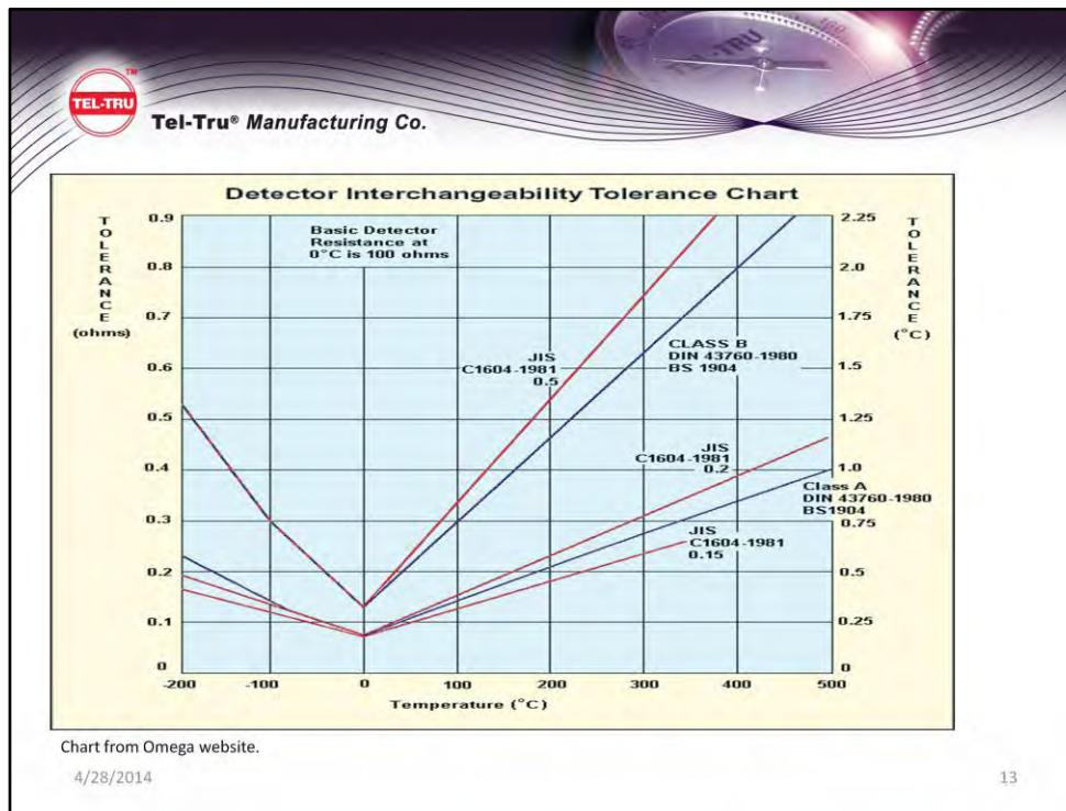
RTD sensors are specified according to their resistance in ohms at zero degrees Celsius. A PT100 element measures 100 ohms at 0° C . The electrical resistance measured in ohms increases as temperature increases. Prompting a repeatable resistance versus temperature relationship.
