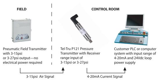
The Tel-Tru P121 is available in a wide range of configurations for converting pneumatic signals to electronic outputs that will allow interfacing with newer electronic systems. These types of applications may be found in a broad range of markets, including chemical processing, petroleum refining, steel milling, and water/wastewater treatment.
