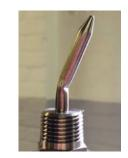
A bend in the probe will limit movement of the internal parts
