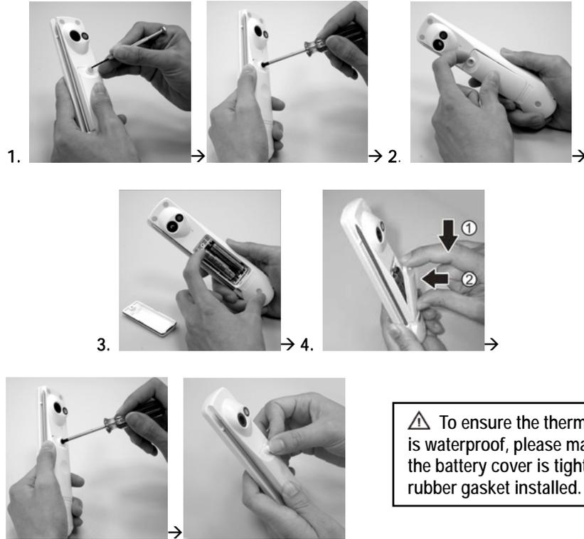
**⚠ To ensure the thermometer is waterproof, please make sure the battery cover is tight with the rubber gasket installed.**
